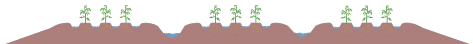
Cross-section view of finished system with drainage canals, basins with furrows, and planted beds
